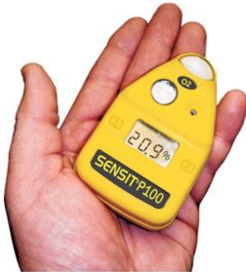
Single gas meters for CO and O2 can provide additional protection for the technician during testing.
